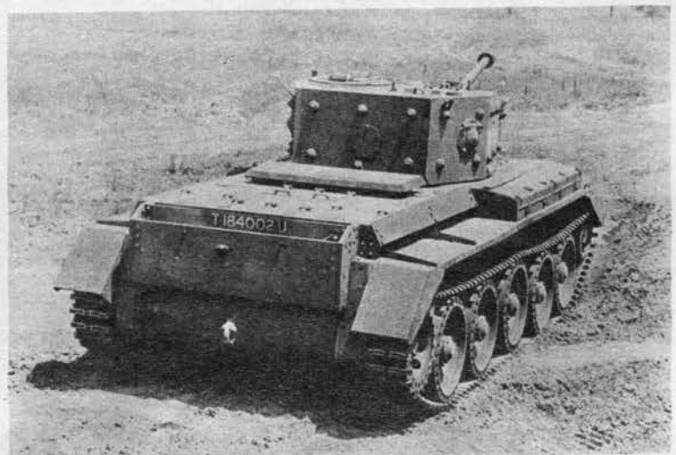
British Cromwell tank is unique-looking with its low, flat-topped hull and straight-sided, heavily-bolted turret. Its six-pounder main gun is the heaviest British tank armament. Suspension resembles T-34's.
